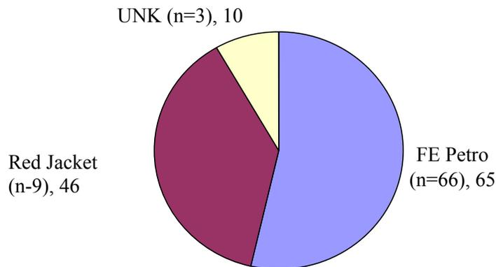
For the 3-gal/hr leak rate, a substantial difference in performance was found associated with turbine manufacturer. This is illustrated in Figure 3.2.3b, which shows the detection rate by simulated leak rate and by turbine manufacturer. Note that for the 3-gal/hr leak rate, the detection rate was 85% for ELLDs with Red Jacket turbines but considerably less, 58%, with FE Petro turbines. This difference was statistically significant at the 5% significance level.
