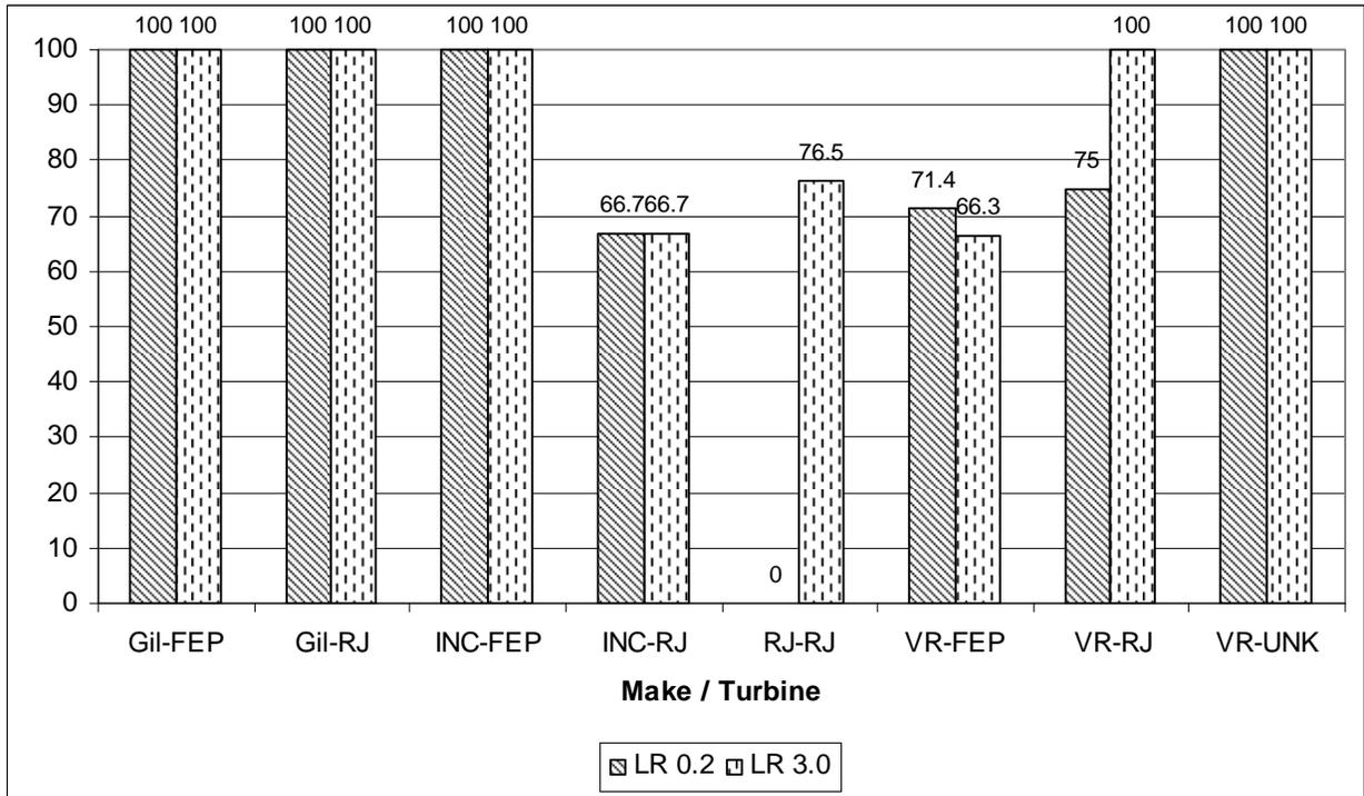
As noted in the body of the report, the difference in 3-gal/hr detection rates for Veeder-Root seems to be a result of a problem with a part in FE Petro turbine pumps. The data are displayed in Table I-6.
