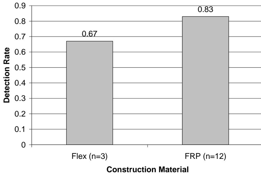
Figure I-5. ELLD Detection Rate at 0.1-gal/hr, by Single- or Double-Walled Pipe
