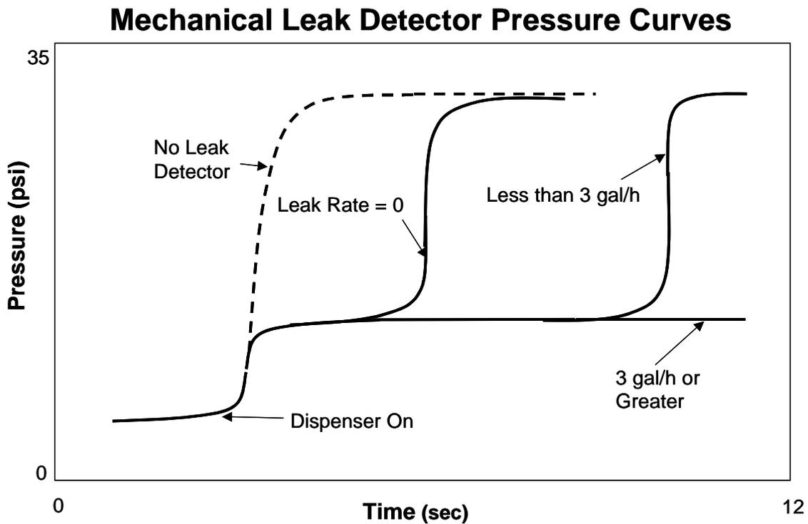
Step one occurs when the dispenser is activated. The pressure rises rapidly to the metering pressure of around 10-20 psi. The flow rate during this step is approximately 3-gal/min.
